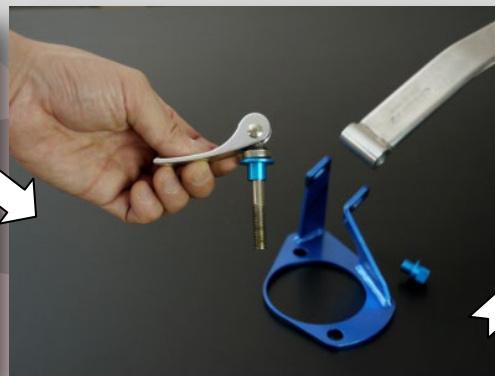
Insert Quick Release Lever and hand-tighten.
