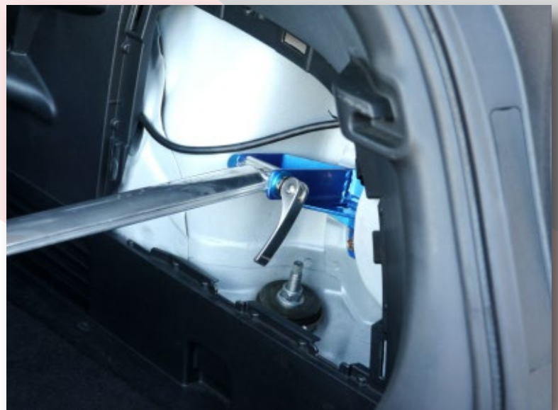
Insert Quick Release Lever and hand-tighten.
