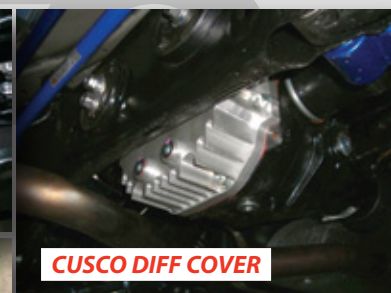
Tapped For External Oil Cooler
