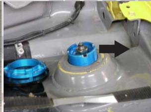
Suspension assembly is simply passed through the strut hole
