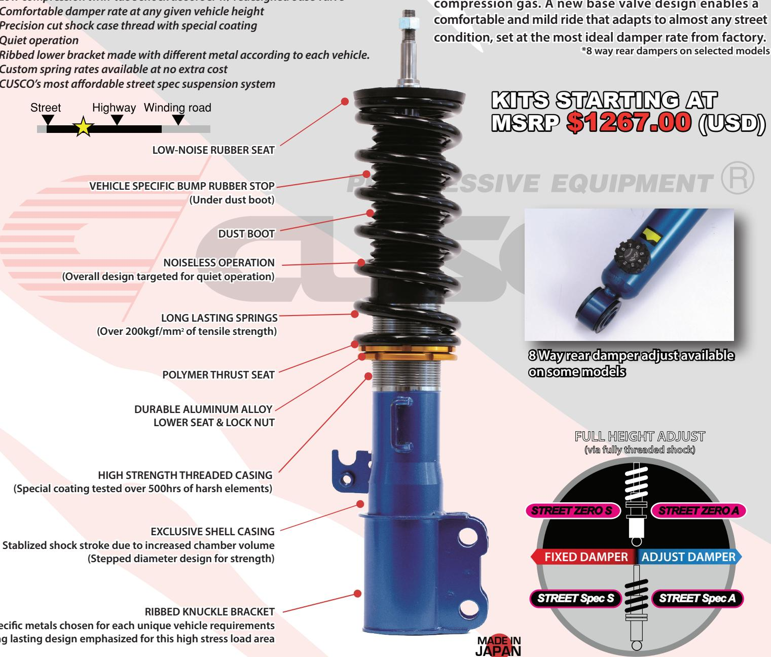
The newly developed twin tube shock absorber features a virtually noiseless design due to its internal low compression gas. A new base valve design enables a comfortable and mild ride that adapts to almost any street condition, set at the most ideal damper rate from factory.
