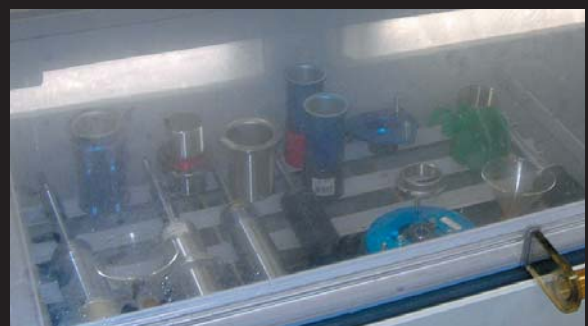
High concentration saltwater direct injection test
