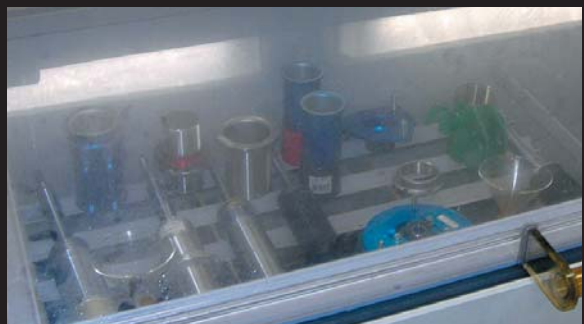
High concentration saltwater direct injection test
