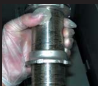
Outside thread of shock body case - After test
