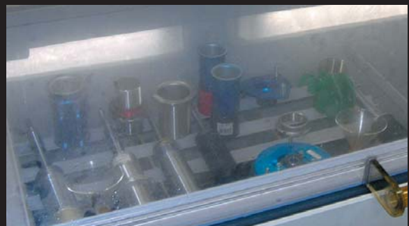
High concentration saltwater direct injection test
