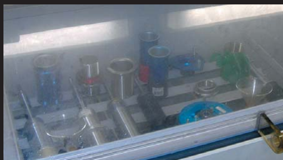
High concentration saltwater direct injection test
