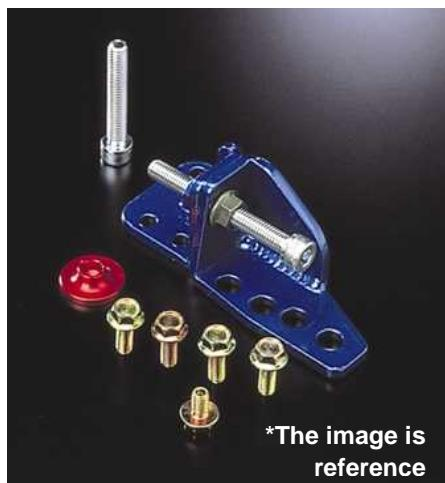
B.C.S. is reinforcement parts for master cylinder to save deflexion on bulk head when its breaking. With fitting on tip of brake master cylinder, breaking feeling will be changed to more direct.
