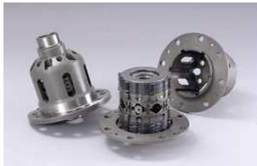
There are two type of differential; Type-RS takes initial torque by coil spring while Type-MZ takes by cone plate.
