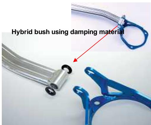
New oval section shape, aluminium made shaft
