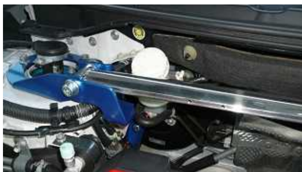
Fitting with tighten together with Shaft of Tower bar and Bracket
