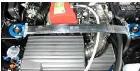
With fitting Strut tower bar, not only body rigidity is improved, but also it affect on better suspension performance.
