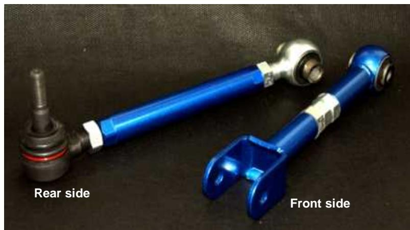
This product adjust camber with low-down to proper angle. It improves unstable movement and prevents offset wear of tyres. Also traction will be improved due to consistent ground of tyres.
